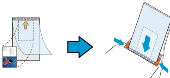
2. Load the Carrier Sheet with the gray section (printed section) facing downwards.
