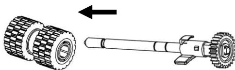
5. Insert the new rollers to the shaft.
