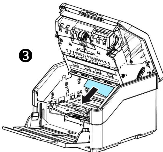
3. Close the ADF by pressing down on the center of the ADF to return it to its original position until it clicks into place.
