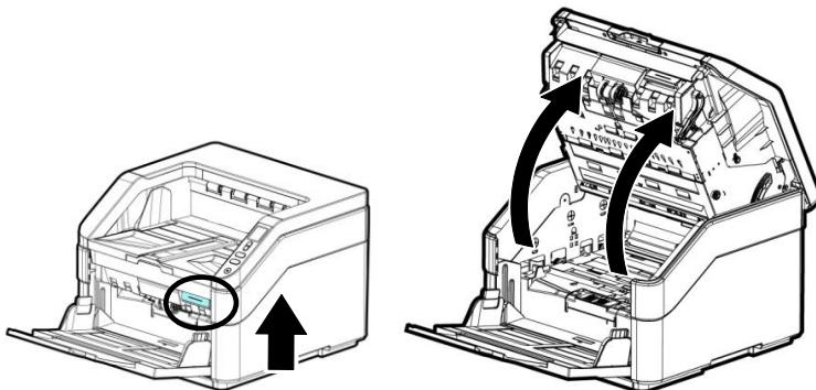
2. Carefully pull the paper out of the ADF unit.
