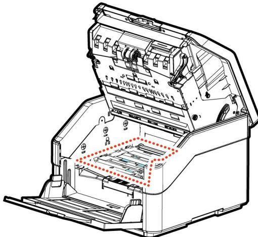
5. When the cleaning is done, press the [**Scan**] button, the feeding roller will be rotated a little automatically.
