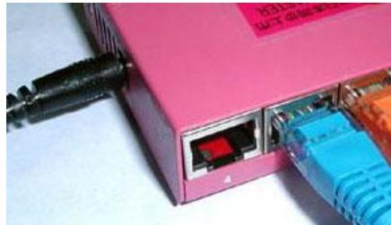
2. Connect the other end to the LAN port marked
