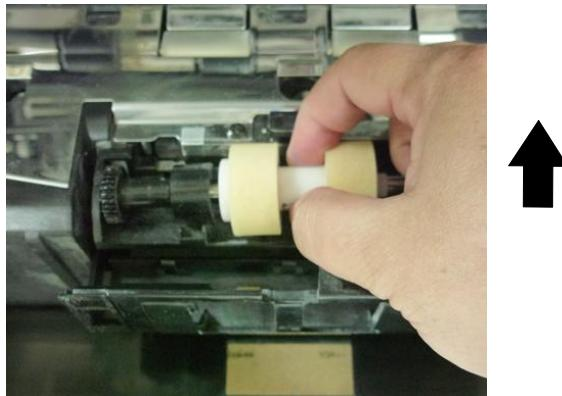
4. Remove the rollers from the shaft.
