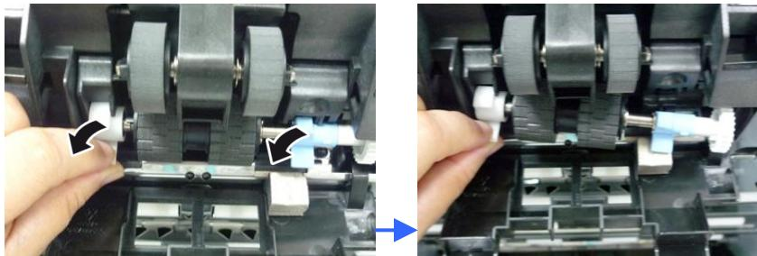
4. Remove the rollers from the shaft.
